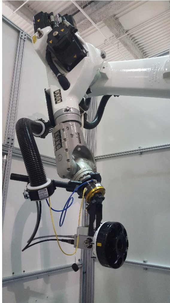
FlawExplorer Shearography System combination with an automated robotic inspection.
