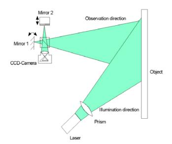
Fig.2: Schematic diagram of a shearography system.
