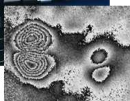
Fig. 1: Phasemap of two impact damages.
