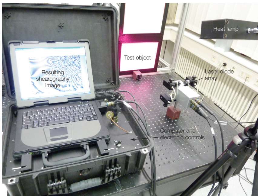
Figure 4. Laser shearography setup for portable camera system.
