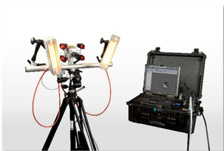
Image 12 The Q-800 Portable Shearography system
