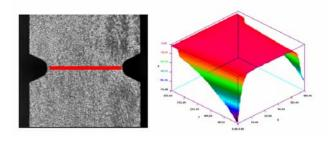
Fig. 5: Variation of the transverse strain as a function of the position across the notch and the measurement steps. The red line indicates the line where the values for the diagram have been taken.
