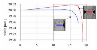
Fig. 7: In-plane movement of the notched specimen at elastic (left) and plastic (right) behavior.
