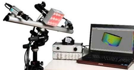
Figure 17 - Q-400 DIC System with two cameras and illumination option
