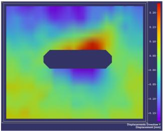
Figure 3: DIC vertical displacement results
