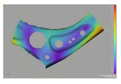
Figure 10 - Two camera DIC measurement limited to surface only, not showing shadowed areas.
