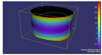
Figure 2 - Full-field evaluation of a cylindrical object with an 8 camera DIC System
