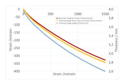
Figure 9 - Thickness changes, strain in thickness and perpendicular to direction of the load
