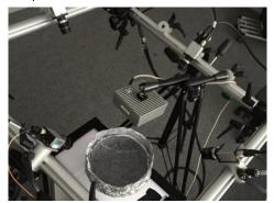
Figure 12 - Setup of multi-camera system for measurement of a hemisphere
