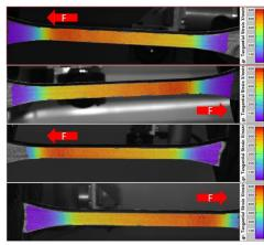
Figure 6 - Front and backside strain in loading direction tensile test sample
