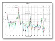
FFT analysis of a component vibration
