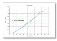
Thermal expansion coefficient (CTE) calculation
