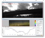
Bridge displacement under load of passing truck
