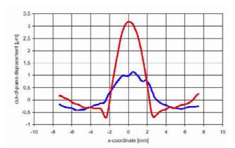
Fig. 7: Out of plane displacement in the diagonal of flip chip assemblies with (soft grey) and without (dark
