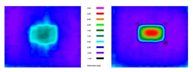
Fig. 6(a): 3D-ESPI out of plane displacement measured between 25°C and 125°C on the assembly from fig. 5 the die is connected with all its bumps. (b): Same measurement for a die with only half of its bumps. The grey scale indicating the z-displacement is the same on both figures.
