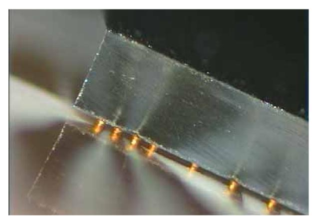
3D-Electronic Speckles Pattern Interferometry (3D-ESPI). This original non contact and full field technique allows deformation measurements of microsystems with a submicron resolution and was successfully applied to detect defaults such as missing bumps in flip chip assemblies.
