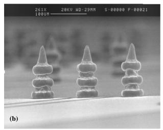
Fig 1: Simple (a) and triple stacked (b) stub bumps.
