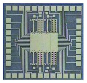
Fig. 5: Flip chip assembly (GaAs die connected on AlN substrate) for 3D ESPI measurements
