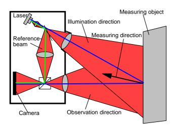
Fig. 3: Basic principle of an ESPI set-up
