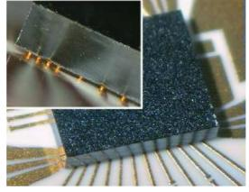
Fig. 2: Top and side (inset) view of a flip chip assembly.
