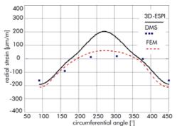
Fig. 9: Shear tensile specimen, cross bar 3 mm: radial strain at 5.6 mm distance, comparison with strain gauge measurement and FEA
