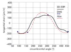
Fig. 8: Shear tensile specimen, cross bar 9 mm: tangential strain at 4.3 mm distance, comparison with strain gauge measurement and FEA
