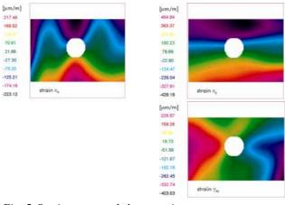
*Fig. 5: Strains*  $\varepsilon_{y}$ *,*  $\varepsilon_{y}$  *and shear strain*  $\gamma_{xy}$
