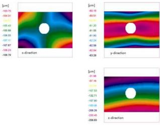
Fig. 4: Deformation components of the shear tensile specimen with 9 mm crossbar
