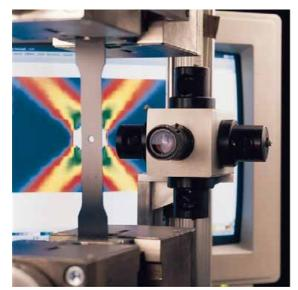
Fig. 1: 3D-ESPI-system for deformation and strain analysis in a tensile testing machine. The figure shows the strain distribution on a tensile specimen with central hole.
