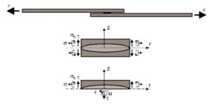
Fig. 2: Structure of a shear tensile specimen
