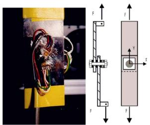
Fig. 3: View of a shear tensile specimen with simulated spot weld. The drawing shows the coordinate system and the measuring field for a specimen with 9 mm cross bar similar to a bolt or rivet.
