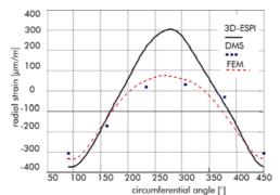
Fig. 7: Shear tensile specimen, cross bar 9 mm: radial strain at 5.6 mm distance, compared with strain gauge measurement and FEA
