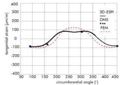
Fig. 10: Shear tensile specimen, cross bar 3 mm: tangential strain at 4.3 mm distance, comparison with strain gauge measurement and FEA
