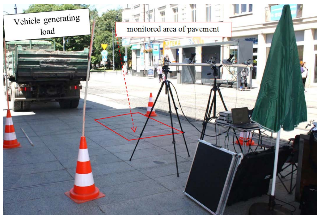
Figure 7. Test stand during DIC deflection measurements of block element pavement structure.
