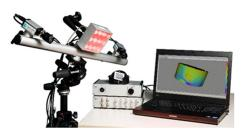
Image 6: Q-400 DIC System with two cameras and illumination option
