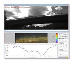
Image 4: Load test results - truck passing bridge
